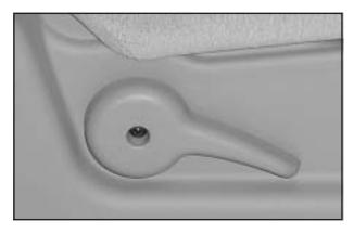
If you have manual reclining seatbacks, the lever is located on the outboard side of the seat cushion. To adjust the front seatback, lift the lever. Release the lever to lock the seatback where you want it. Lift the lever without pushing on the seatback and the seatback will go to an upright position.
